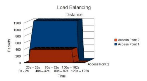
Figure 2: Same Rates - Distance algorithm (full time experiment)
