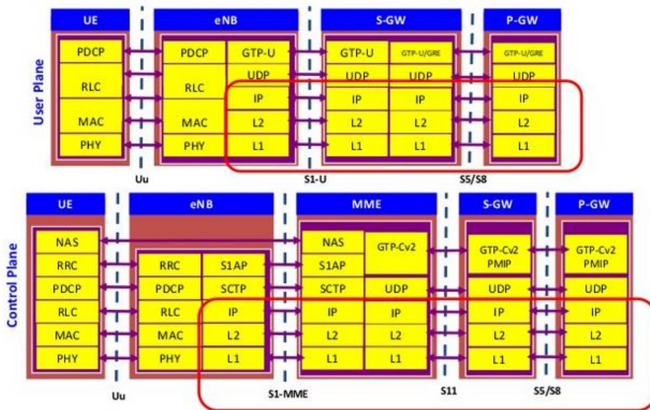
Figure 25. Control and User Plane in LTE [A].
