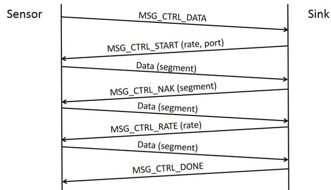
**Figure 4.3:** Data exchange stage.
