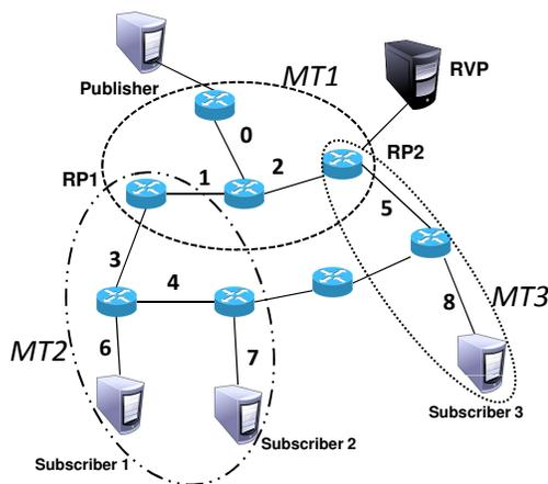
**Figure 2.2:** An example of a multicast tree with relay points.
