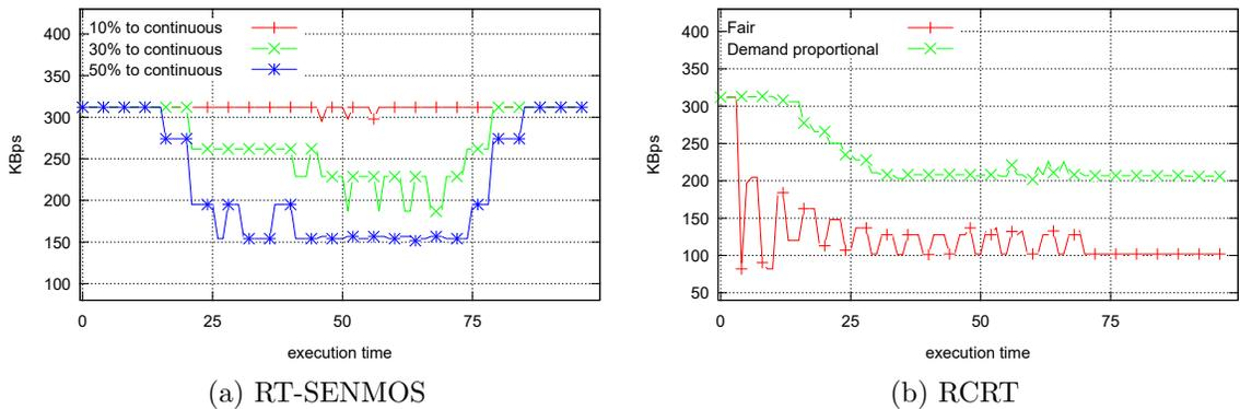
**Figure 4.13:** Mixed sensor scenario - Mean Bandwidth Allocated to event sensors (2% loss).
