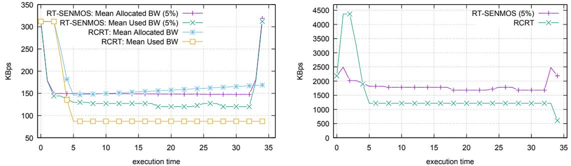
(a) Mean Bandwidth Usage - RT-SENMOS (b) Total Bandwidth Usage - RT-SENMOS vs RCRT
