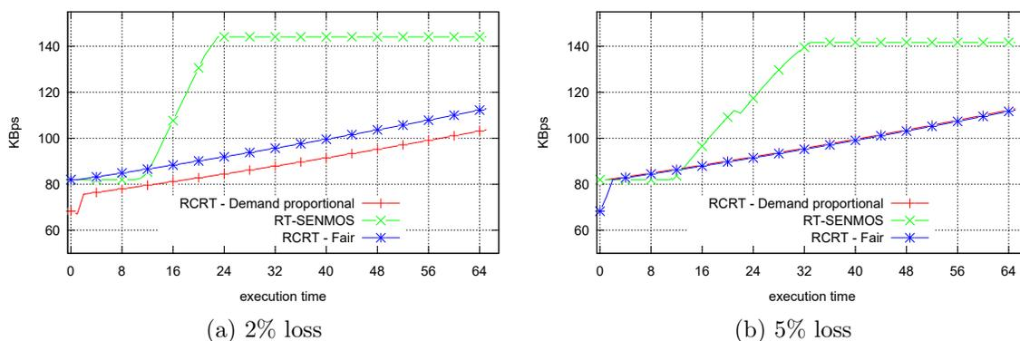
**Figure 4.10:** Continuous sensor scenario - Mean Bandwidth Allocated to sensors.
