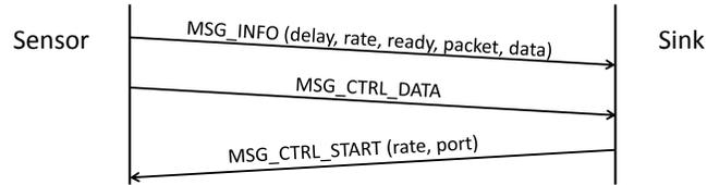
**Figure 4.2:** Start of data exchange stage.
