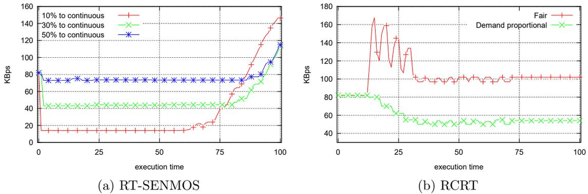
**Figure 4.12:** Mixed sensor scenario - Mean Bandwidth Allocated to continuous sensors (2% loss).
