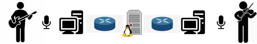
Figure 5.4: Topology using an NMP server.
