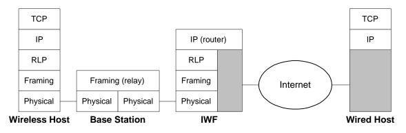
Fig. 1. Connectivity between cellular links and the Internet
