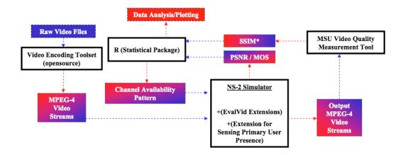
Figure 1. Simulation Testbed.
