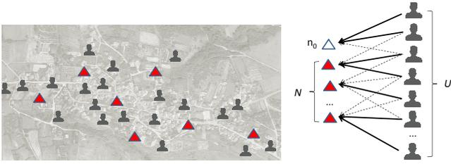
Figure 1: Example physical system layout and options available to CN users under the collective subscriptions' scheme. Each user may join the collective subscription of one node out of a subset of the  $N$  CN nodes or abstain (*i.e.*, “join node  $n_0$ ”).
