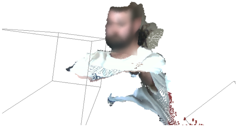
Fig. 3.2: Point cloud rendered with blurred faces. The bounding box demonstrates we can also add 3D detection.
