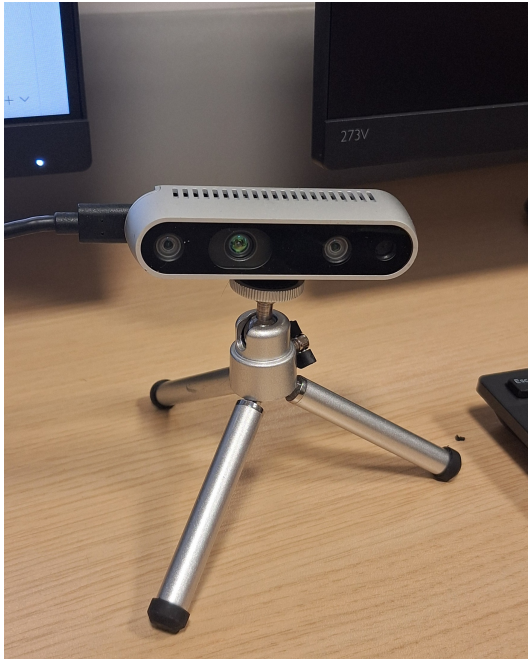
Fig. 2.1: Intel Realsense stereo-depth camera, model D435I
