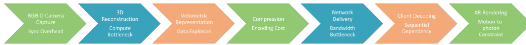
Fig. 1.1: High-level overview of the real-time volumetric streaming pipeline and its primary latency sources. The system focuses on RGB-D capture and interactive 6DoF consumption on resource-constrained XR devices, highlighting the key computational and communication bottlenecks across stages.
