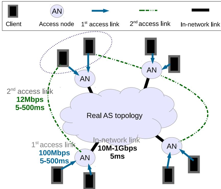
**Figure 4.15:** AS-scale topologies: client attachment to the Access Nodes (AN) of the AS with two access links. The testbed allows configuring different access links' latencies (per user) and in-network link capacities (per experiment).
