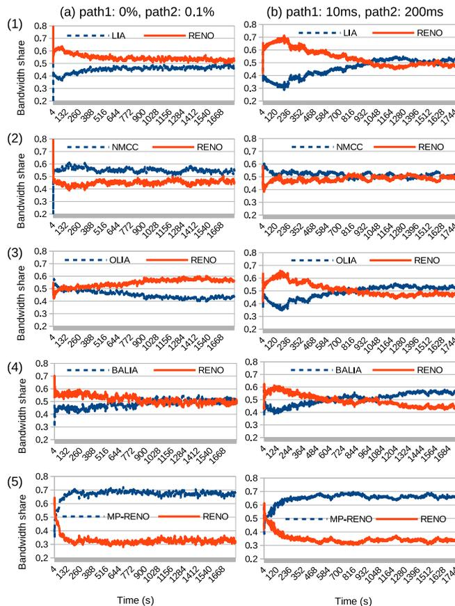
**Figure 5.5:** MPTCP performance in the LAN testbed with two disjoint paths, different congestion algorithms (rows 1-5) and mismatched paths in terms of error-rate (column a) and RTT (column b).
