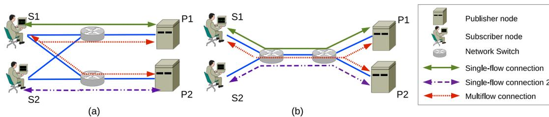
**Figure 4.10:** LAN testbed topologies for assessing performance in (a) disjoint paths and (b) paths with shared bottlenecks.
