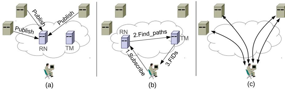
**Figure 4.1:** mmTP operation phases: (a-b) slow-path rendezvous, where connection is established, and (c) fast-path rendezvous, where data transfer takes place.
