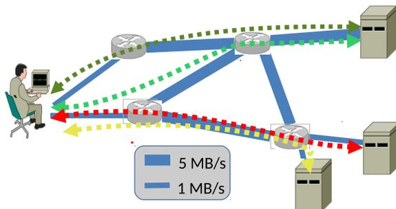
**Figure 3.1:** An example of multiflow transfer where two paths (multipath) are established to two content sources (multisource), thus deploying four paths in total.
