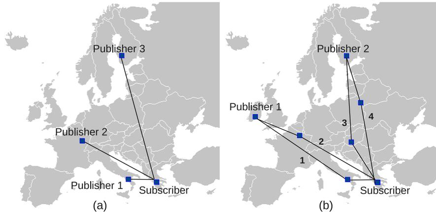
**Figure 4.4:** PlanetLab overlay topologies that allow (a) multisource with three content sources and (b) multiflow with two content sources and two paths to each source.
