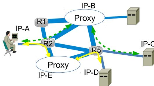
**Figure 3.6:** An example of multipath transfer in the TCP/IP architecture based on overlay routing. The single-homed endpoints communicate through two intermediate relay points, thus forcing multipath delivery with enhanced path diversity. Often overlay networks are combined with other techniques, such as multihoming with SOCKS servers [2] and multisource, as presented in this figure.
