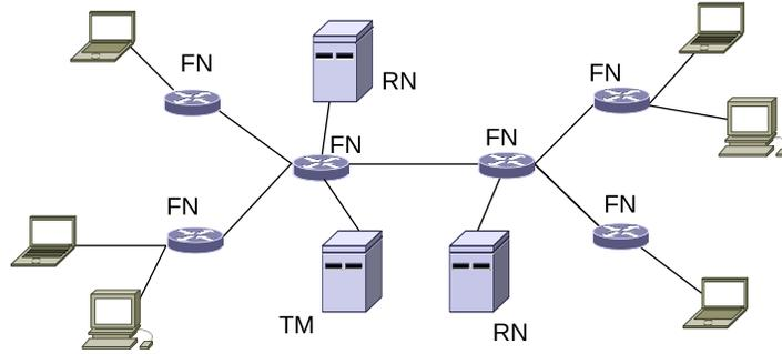
**Figure 2.1:** A PSI network consisting of Forwarding Nodes (FN), Rendezvous Nodes (RN), a Topology Manager Node (TM) and hosts.
