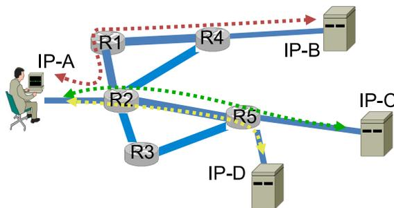
**Figure 3.2:** An example of multipath transfer in the TCP/IP architecture based on multisource. The single-homed receiver associates its address with the addresses of many single-homed content sources, in order to deploy multiple end-to-end connections.
