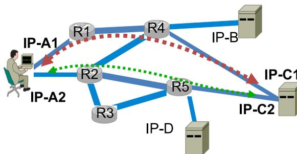
**Figure 3.3:** An example of multipath transfer in the TCP/IP architecture based on multihoming. The multihomed receiver uses two IP addresses to deploy two end-to-end subflows with the multihomed content source.
