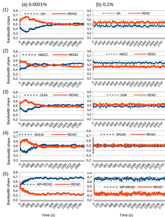
**Figure 5.4:** MPTCP performance in the LAN testbed with two disjoint paths, different congestion algorithms (rows 1-5) and different packet drop rates (columns a,b).
