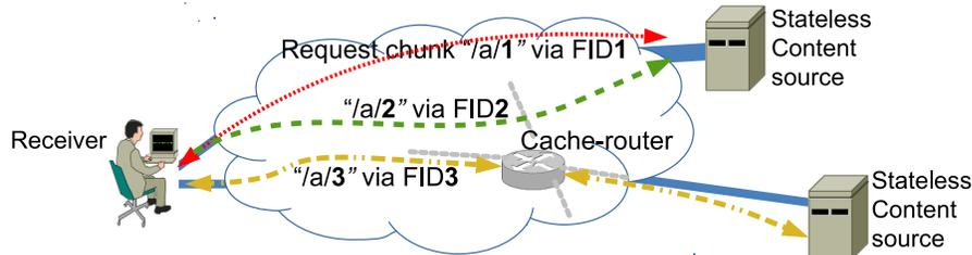
**Figure 4.2:** mmTP operation during fast-path rendezvous. FIDs correspond to different paths to the stateless content sources. Data chunks are self-identified through algorithmic identifiers in the form of “/content\_name/chunk\_ranking”, i.e. “/a/1” is the 1<sup>st</sup> chunk of content “a”. The *pull* transfer model and the named data chunks allow distributed on-path chunk-level caching.
