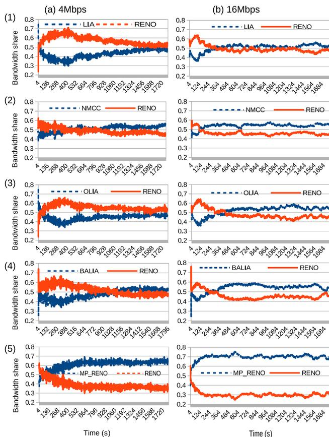
**Figure 5.3:** MPTCP performance in the LAN testbed with two disjoint paths, different congestion algorithms (rows 1-5) and different transfer rates (columns a,b).
