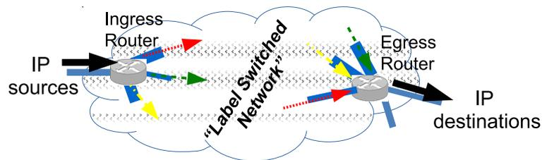
**Figure 3.5:** An example of multipath transfer in the TCP/IP architecture based on the MPLS source routing technique. IP traffic enters the source-routed network via the ingress router that shares the traffic volume among different explicitly defined paths until the egress router. The same approach is followed by most source routing techniques [1, Sect.II.A].
