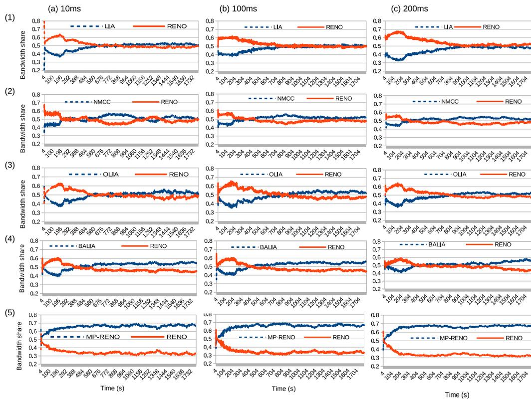
**Figure 5.2:** MPTCP performance in the LAN testbed with two disjoint paths, different congestion algorithms (rows 1-5) and different path latencies (columns a-c).
