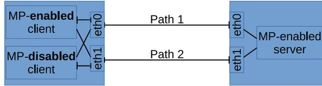
**Figure 5.1:** LAN testbed topology for evaluating MPTCP in Linux. Two client VMs are co-hosted in the same client node.
