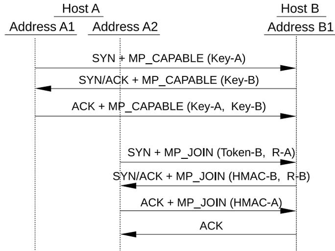
**Figure 3.4:** The two handshakes required for establishing two MPTCP subflows. “R-A/B” are random numbers selected by the hosts to avoid replay attacks. “Token-B”, which is generated from Key-B, is used for authenticating the new subflow. “HMAC-A/B” are the *Hash-based Message Authentication Codes* (HMACs) of the hosts.
