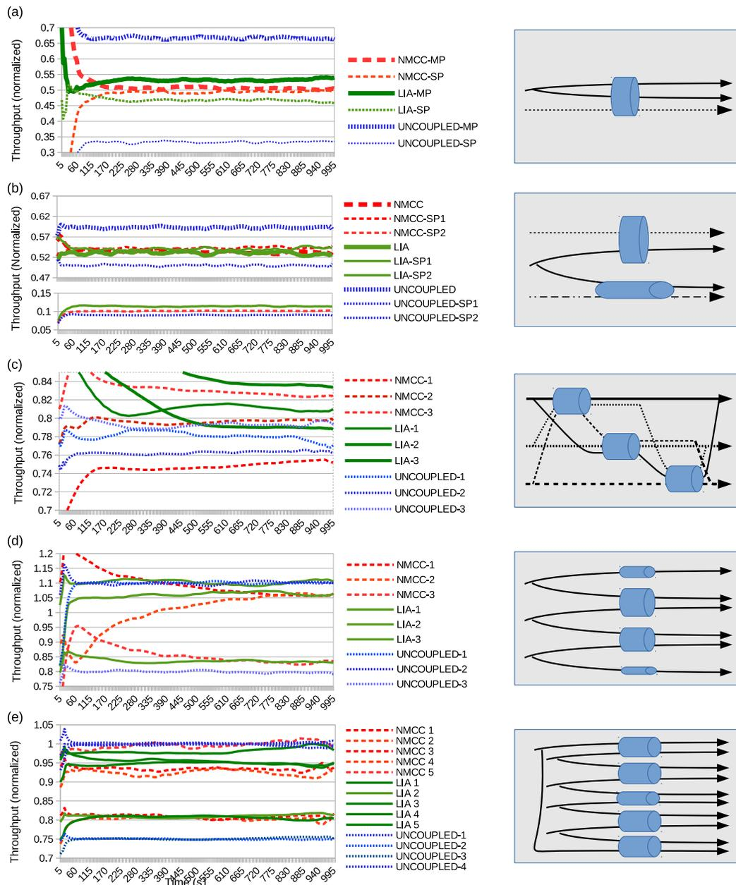
**Figure 4.14:** LIA and NMCC performance comparison (left column) in the benchmark topologies of [3] (right column). Figures illustrate the instant bandwidth share of multipath (MP) and single-path (SP) connections normalized to the overall network capacity unless otherwise stated. Figure (a) examines NMCC’s efficiency in terms of TCP-friendliness, (b)-(c) resource utilization and (e)-(d) load balancing.
