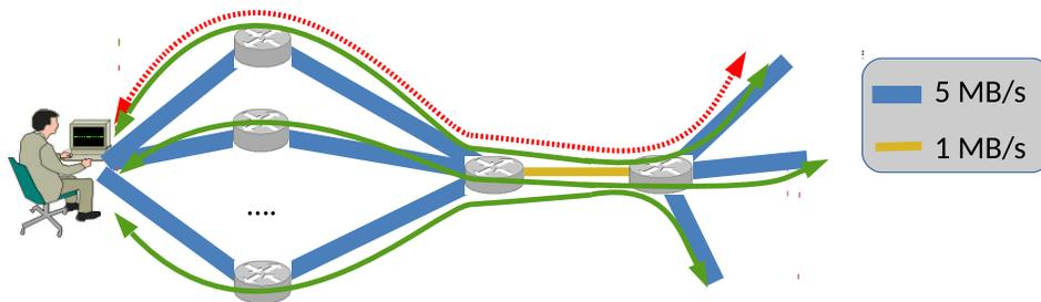
**Figure 3.7:** An example of the TCP-friendliness issue. The single-path connection (red dashed line) gets  $1/(N + 1)$  MB/s when competing in the same bottleneck (yellow link) with a multiflow connection of  $N$  subflows (green lines). Notice, that the issue is independent of the number of exploited sources, thus concerning multisource and multipath in general.
