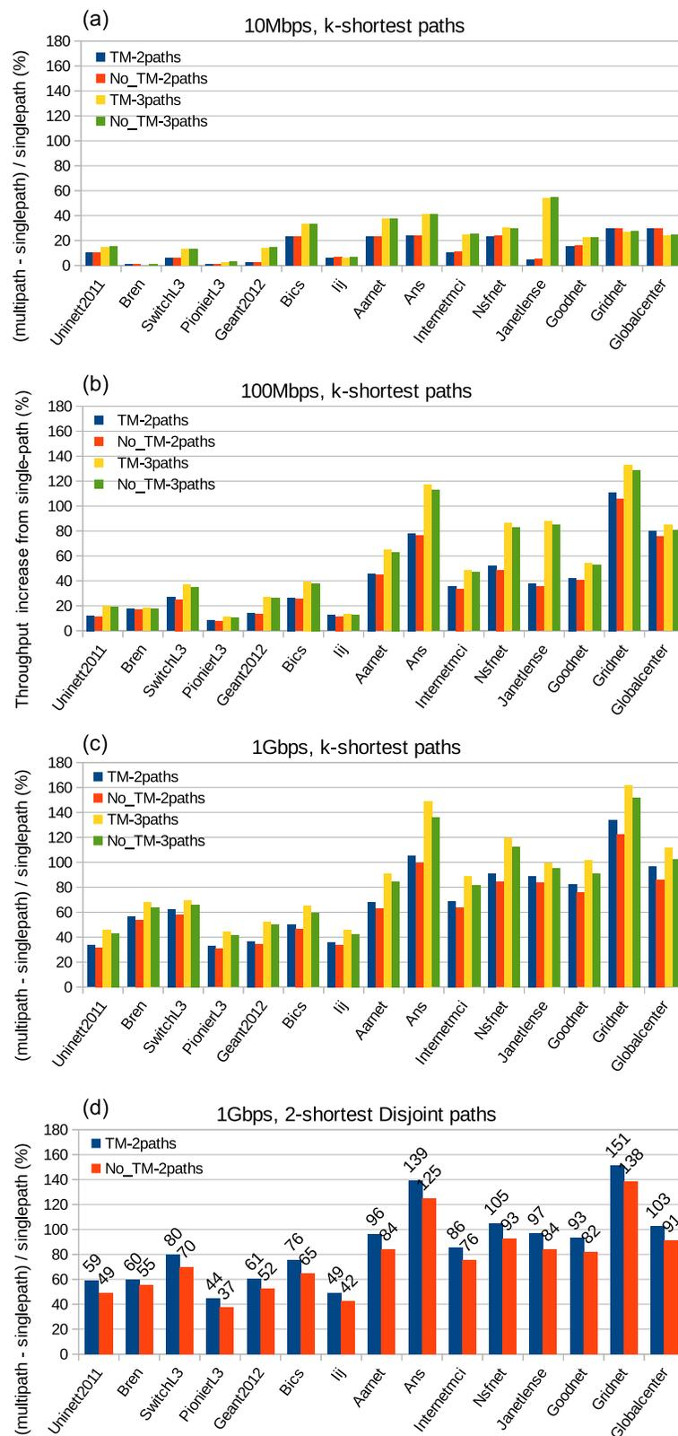
**Figure 4.17:** mmTP performance in the domain-scale topologies with and without TM assistance under different path formation policies and in-network link capacities: (a-c) Yen’s path formation algorithm and (d) Bhandari’s disjoint path formation algorithm. Topologies are plotted in ascending order by density from the left to the right.
