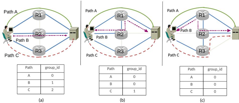
**Figure 4.8:** An example of TM assistance in three different cases of path composition: (a) Disjoint paths, (b) two paths sharing one link, (c) three paths sharing two links.
