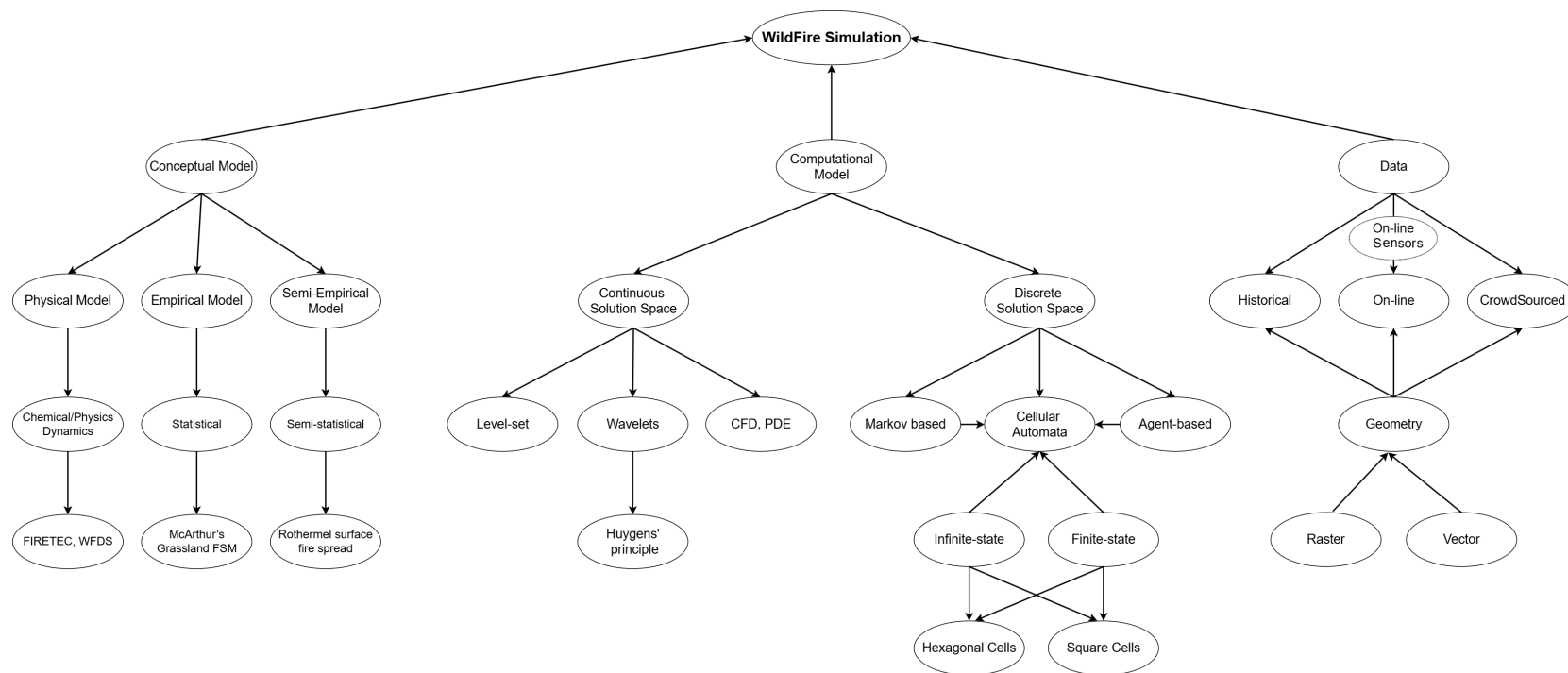
Figure 2.1: A comprehensive taxonomy of wildfire spread and simulation methods. Adapted from [15].
