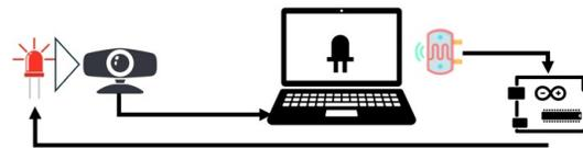
Fig. 6. Topology for local LED-based video latency measurements.
