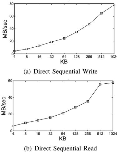
Fig. 10. I/O Throughput in a large deployment
