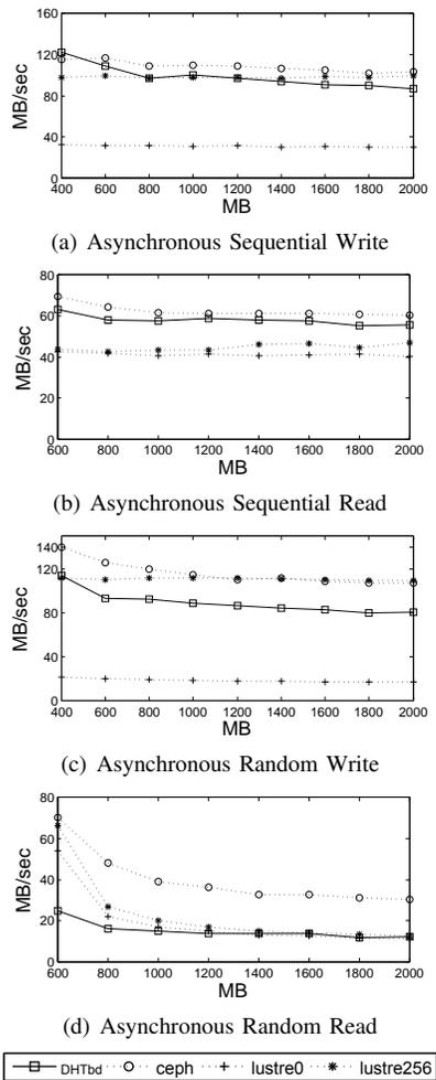
Fig. 6. I/O Throughput Comparison (AIO)
