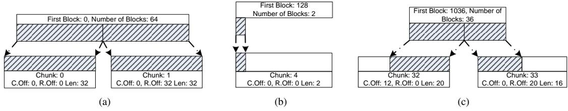
Fig. 2. Mapping blocks to chunks: 1<sup>st</sup> request (a) , 2<sup>nd</sup> request (b) , 3<sup>rd</sup> request (c)
