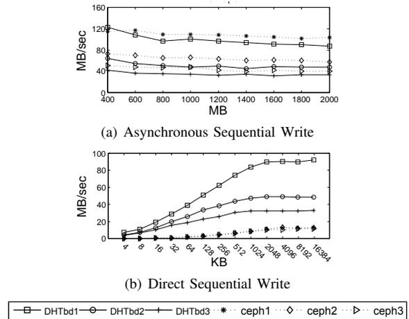
Fig. 11. I/O Throughput for various replication levels
