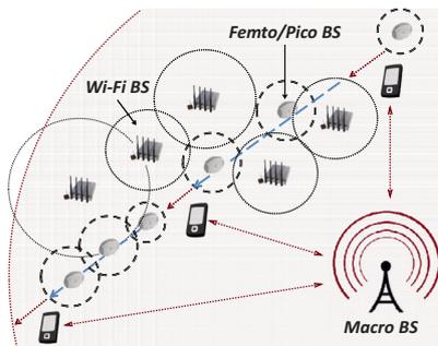
**Fig. 2.** Macro-cellular area including provider's pico/femto cells and third-party Wi-Fi hotspots. Blue-dashed (resp. red-dotted) arrows denote that the mobile is connected to a small (resp. the macro) BS.
