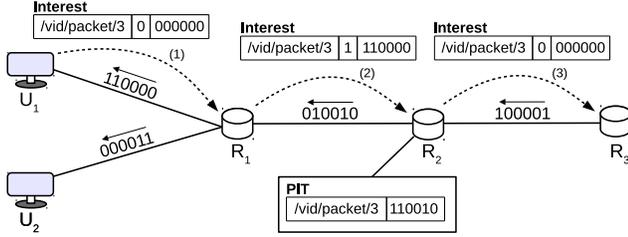
Fig. 4. Interest from  $U_1$ :  $R_1$  updates the Interest iBF.  $R_2$  tracks the Interest with the iBF for  $R_2 \rightarrow R_1 \rightarrow U_1$ .  $R_2$  resets the iBF to 0 and forwards the Interest.
