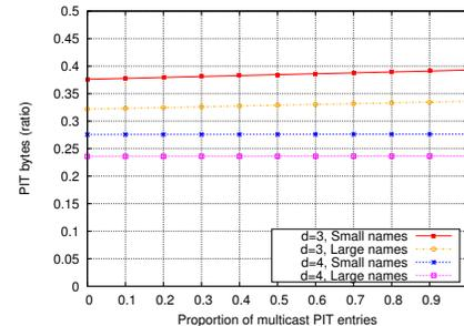
Fig. 14. PIT size reduction (in bytes) depending on the fraction of multicast Interests.
