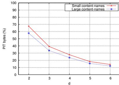
Fig. 12. PIT size reduction (in bytes) for small (20-bytes) and large (56-bytes) content names (Zipf group sizes).
