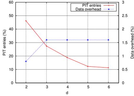
Fig. 7. PIT entries and Data overhead for unicast traffic as a function of  $d$ .
