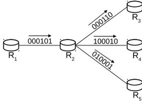
Fig. 3. Bloom filter-based forwarding. Links are annotated with LIDs ( $m = 6$  and  $k = 2$ ).
