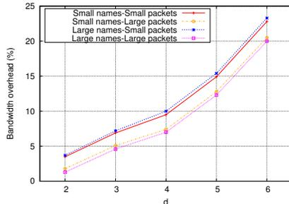
Fig. 13. Bandwidth overhead for small (36-byte Interests) and large content names (70-byte Interests), with small (1500 bytes) and large (7500 bytes) Data (Zipf group sizes).
