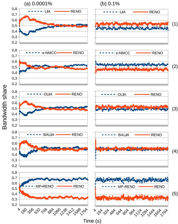
Fig. 5. MPTCP performance in a LAN with two disjoint paths, different congestion algorithms (rows 1-5) and packet drop rates (columns a-b).
