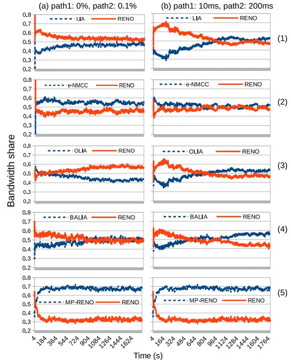
Fig. 6. MPTCP performance in a LAN with two disjoint paths, different congestion control algorithms (rows 1-5) and heterogeneous paths in terms of error-rate (column a) and RTT (column b).
