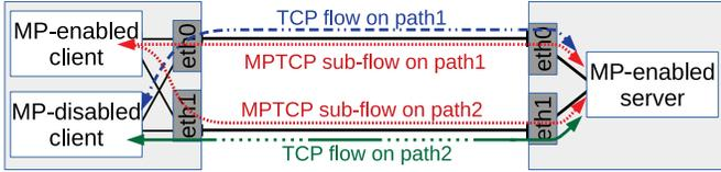
Fig. 2. Experimental topology for evaluating MPTCP in Linux. Due to space constraints, we plot only one MPTCP connection and two TCP connections; in the experiments we deploy four MPTCP and four TCP connections in total.
