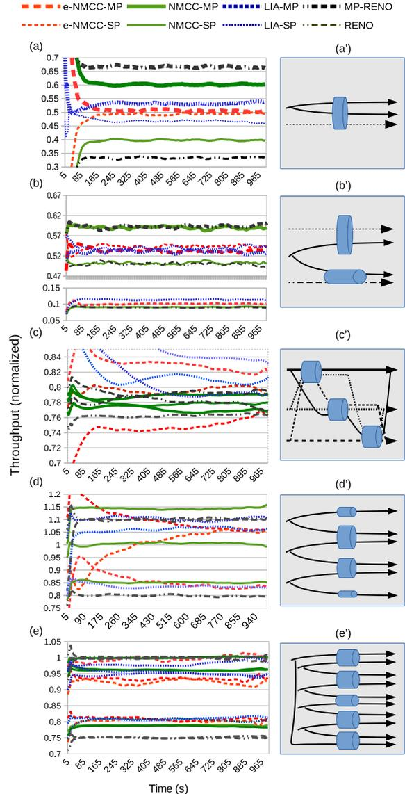
Fig. 9. MPTCP performance in the benchmark topologies of [8]. Figures illustrate the instant bandwidth share of multipath (MP) and single-path (SP) connections normalized to the overall network capacity, unless otherwise stated. Figure (a) examines TCP-friendliness, (b)-(c) resource utilization and (e)-(d) load balancing.
