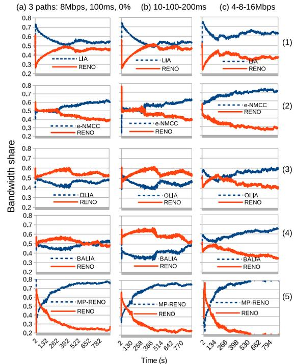
Fig. 8. MPTCP performance in a LAN with three disjoint paths, different congestion control algorithms (rows 1-5), identical paths (column a) and paths differing in latency (column b) or bandwidth (column c).
