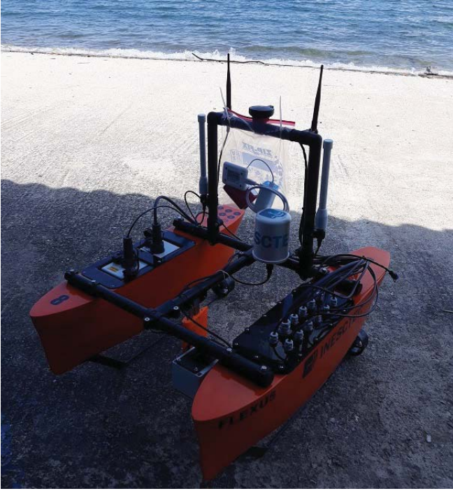
Fig. 3. One of the USVs used in the experiments. Note the zip-locked clear plastic bag containing a wireless node hanging from the upper horizontal bar.
