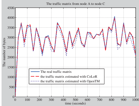
Fig. 6. The real and estimated traffic matrix in the second scenario.
