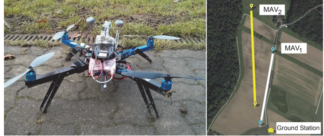
Figure 1: Left: Arducopter platform with on-board wireless package and two external circular antennas. Right: Test scenario of two quadcopters moving between two waypoints: distance of MAV 2 to the ground station varies from 40 – 450 m; distance of MAV 1 to the ground station varies from 20 – 260 m.
