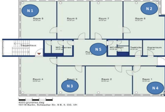
Figure 4: Floor plan for measurement campaign in Berlin consisting of five Lenovo Thinkpad X210T laptops.
