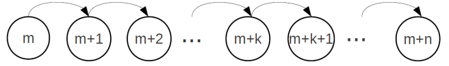
Figure 1: Markov Chain for the dissemination of a content with initial popularity and availability n and m , respectively.
