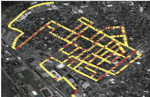
Figure 2: Overhead view of Cambridge, Mass., with satellite link conditions overlaid on roads [1]. Yellow: unblocked. Red: blocked.
