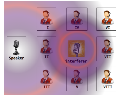
Figure 1: wireless conferencing scenario consisting of 8 listeners, 1 speaker, and 1 interferer.
